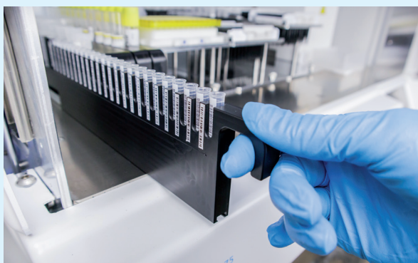
Primary tube handling, the onboard barcode reader and bidirectional connection with the LIS ensure complete traceability
